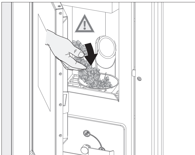
Fig. 2.19 Pour pellets in manually if the pellet duct is empty
