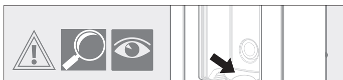
Fig. 3.3 Burner trough visual inspection
