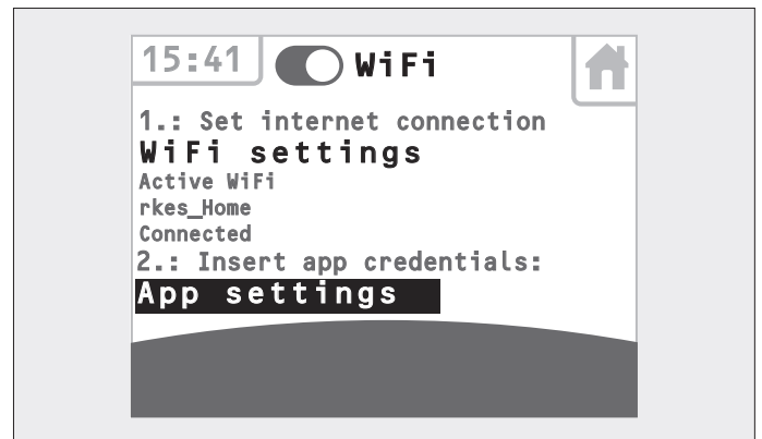
Fig. 3.34 Touch control panel – Wi-Fi receiver switched on
